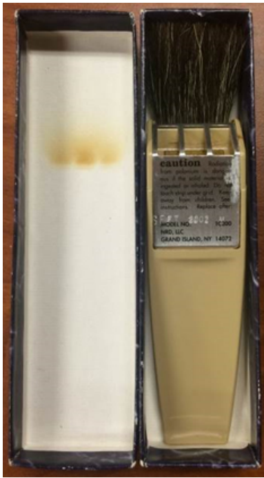
Static eliminator: polonium-210 on bar at the base of the brush. Notice the results of the alpha interactions on the lid of the box after close and continuous exposure. Photo courtesy of Steve Sugarman
